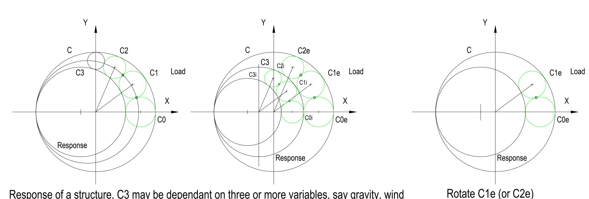
Response of a structure, C3 may be dependent on three or more variables, say gravity, wind and earthquake loads each having a , C0, C1 and C2. The combined area C0, C1, C2 .... shall be equal or as close to C3 as possible. (Left figure above )
