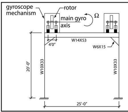
Figure 3: Two mechanisms placed at the support points.
