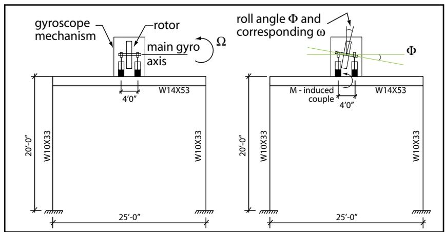
Figure 2 : Steel frame with gyroscope mechanism.
